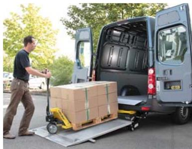
Unfolded the platform provides enough space for loading and unloading a euro pallet with lift truck...
